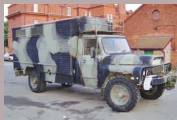
Below left & bottom: Acmat workshop van finished in three-colour camouflage scheme, which had been converted to the field artillery command role. The same vehicle is shown below on exercise in the Glen of Imaal, which has been used for over 170 years as a range. The conversion to this role was a matter of ripping out the Tiffie equipment and using the benches as map tables! Note the aerial mounts on the front bumper, which offer an indication of its true purpose.
