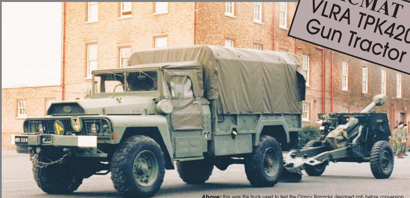
Above: this was the truck used to test the Clancy Barracks designed cab before conversion. Notice the canvas doors that allowed water into the cab as they were not a snug fit.
